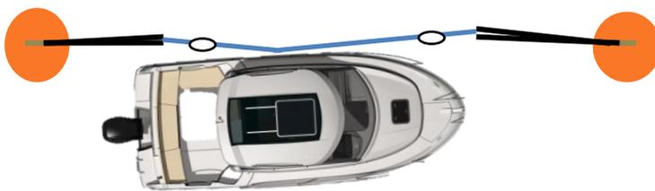
On return to the mooring the floating line can be easily recovered and placed on a midship cleat. Then the rear and front bridle lines can once more be retied forward and aft and pulled up fairly tight to keep the trot mooring in a straight line. It should be noted that manoeuvring a boat back into position must always be carried out at very slow speeds taking account of tide and wind.
